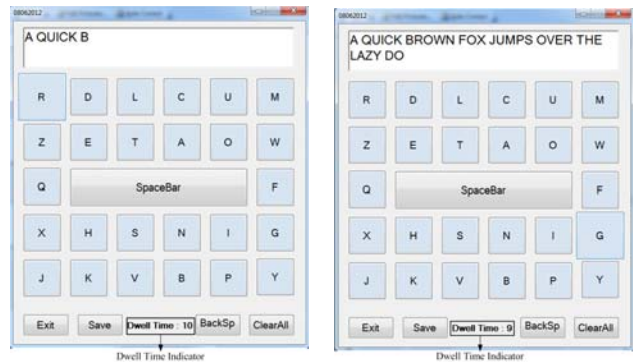
(a) Interface with dwell time 1 second, initially which has been set (b) Depending on the performance of participant, it becomes 900 milliseconds
